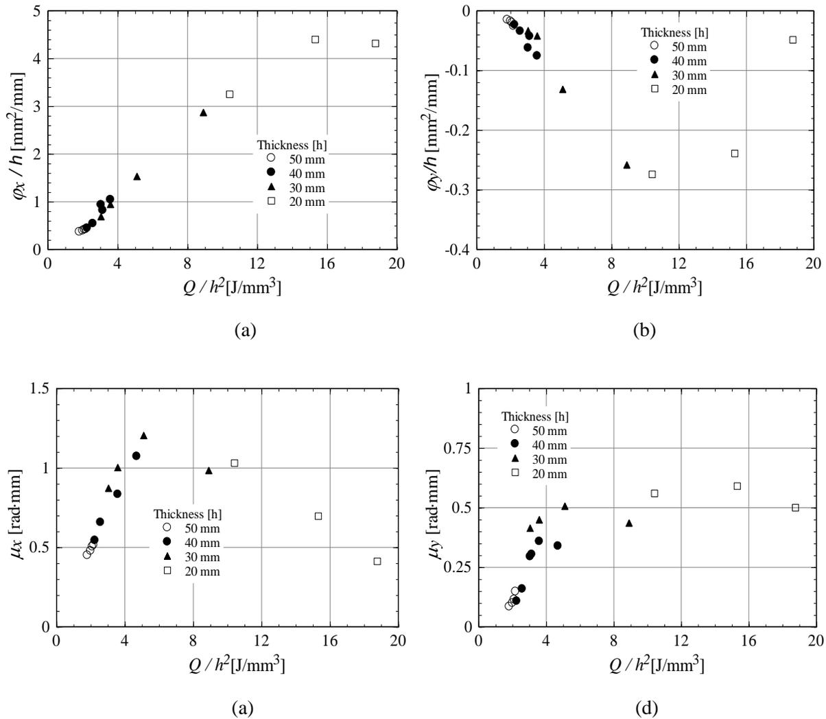
Figure 8 Relation between crossing effect on inherent deformation and heat input parameter  $Q/h^2$
