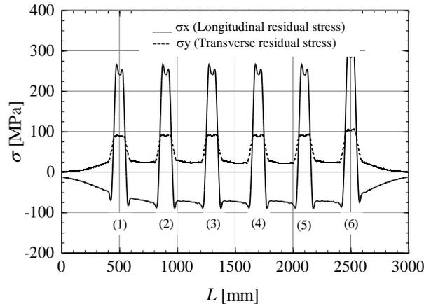
Figure 1 Distribution of residual stresses produced by parallel heating lines spaced 400 mm
