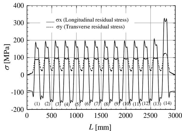
Figure 2 Distribution of residual stress due parallel heating lines spaced 200 mm
