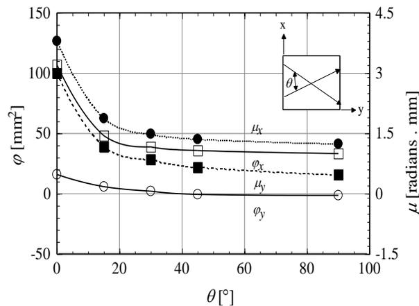
Figure 7 Variation of crossing effect for different angle of intersection between crossed heating lines
