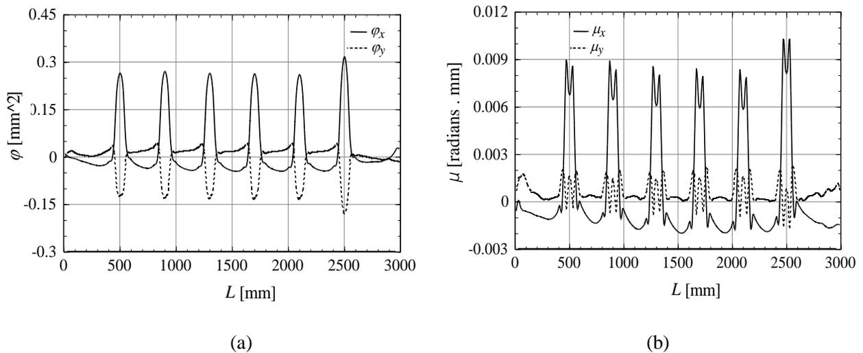
Figure 3 Distribution of crossing effect on inherent deformation for heating lines spaced 400 mm (a) On inherent shrinkage, and (b) On inherent bending
