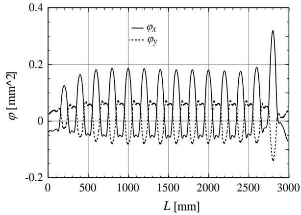
Figure 4 Distribution of crossing effect on longitudinal shrinkage of heating lines spaced at 200 mm
