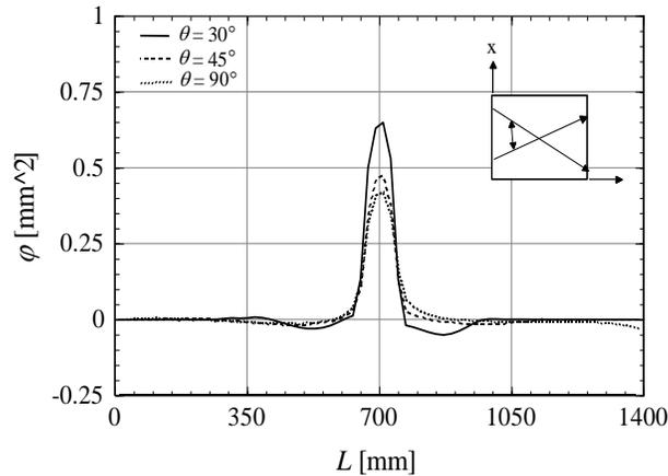
Figure 6 Crossing effect on longitudinal shrinkage
